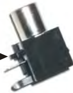
Figure 27. Preparing the RCA Jacks for Installation.
