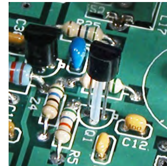
Figure 32. Installing Q1 with Teflon Spacer.
